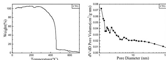
Fig. 2. Ashine CTG Product TGA Analysis and Pore Size Distribution Analysis
